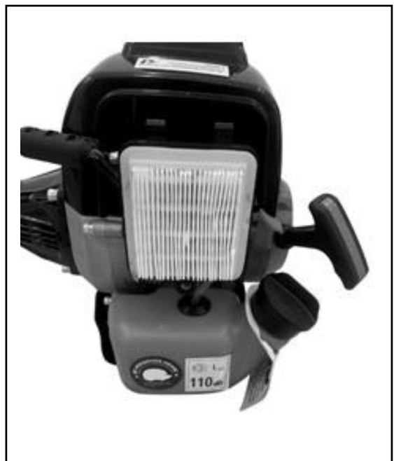
Once the air filter is open, remove the filter to clean and replace when finished.
